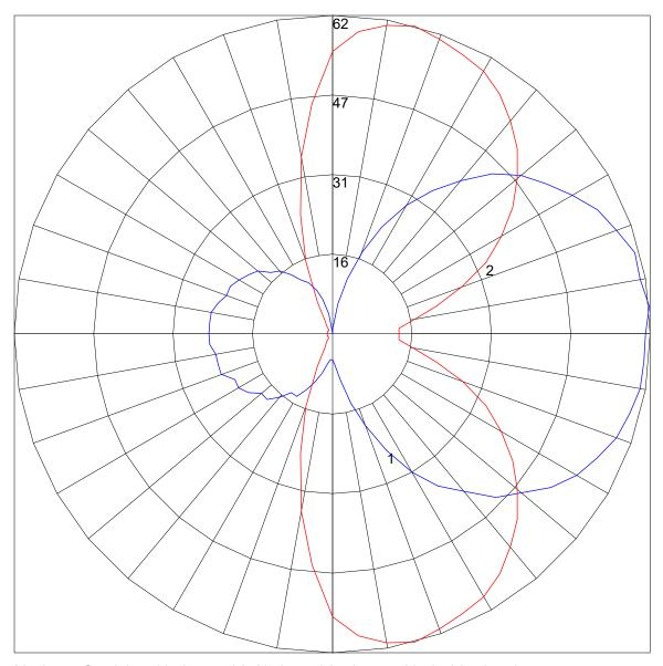
Maximum Candela = 62 Located At Horizontal Angle = 75, Vertical Angle = 95 # 1 - Vertical Plane Through Horizontal Angles (75 - 255) (Through Max. Cd.) # 2 - Horizontal Cone Through Vertical Angle (95) (Through Max. Cd.)
