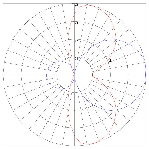
Maximum Candela = 94 Located At Horizontal Angle = 75, Vertical Angle = 100 # 1 - Vertical Plane Through Horizontal Angles (75 - 255) (Through Max. Cd.) # 2 - Horizontal Cone Through Vertical Angle (100) (Through Max. Cd.)
