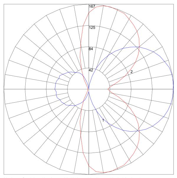
Maximum Candela = 167 Located At Horizontal Angle = 75, Vertical Angle = 95 # 1 - Vertical Plane Through Horizontal Angles (75 - 255) (Through Max. Cd.) # 2 - Horizontal Cone Through Vertical Angle (95) (Through Max. Cd.)
