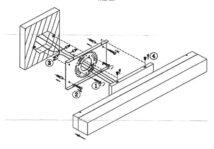
A:Copper ground wire to ground wire-if you only have two wires coming from the electrical box,connect the fixture's copper wire to the green ground screw on the mounting plate.
