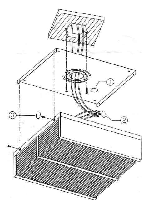
A:Copper ground wire to ground wire-if you only have two wires coming from the electrical box,connect the fixture's copper wire to the green ground screw on the mounting plate.
