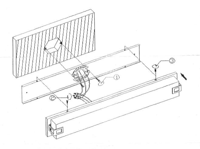
A:Copper ground wire to ground wire-if you only have two wires coming from the electrical box,connect the fixture's copper wire to the green ground screw on the mounting plate.
