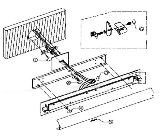
A:Copper ground wire to ground wire-if you only have two wires coming from the electrical box,connect the fixture's copper wire to the green ground screw on the mounting plate. B:White fixture wire to white supply wire.
