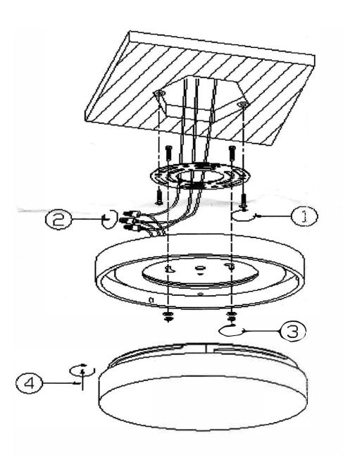
A:Copper ground wire to ground wire-if you only have two wires coming from the electrical box, connect the fixture's copper wire to the green ground screw on the mounting plate.
